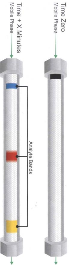
Figure G: Understanding How a Chromatographic Column Works – Bands
