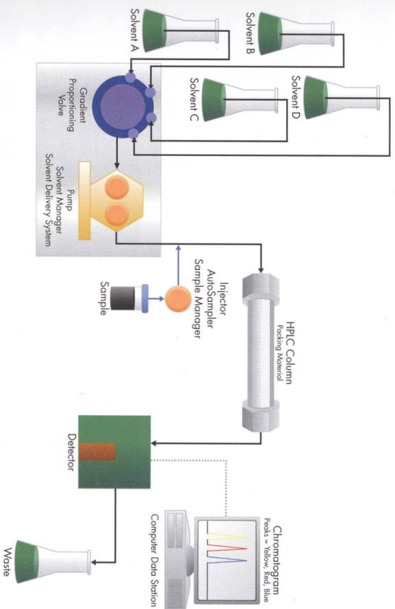
Figure J-3: Low-pressure-gradient System
